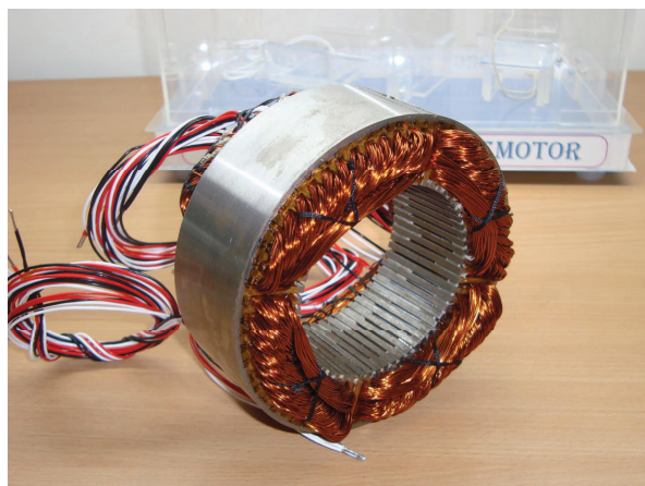
Figure 4.15 60 slots quadruplex winding armature stator
