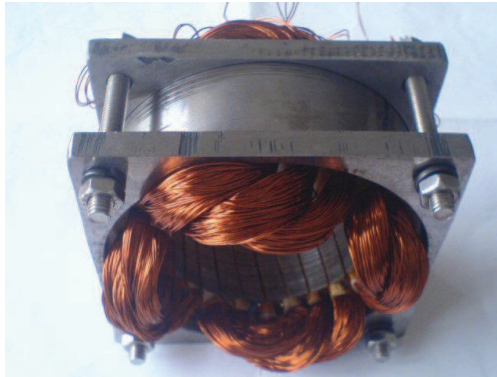
Figure 4.5 24 slots 8 poles armature winding with large overhang
